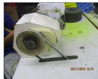
Photo of non-conformity 7.17 Pulley cover of rib cutting machine was displaced.JPG
