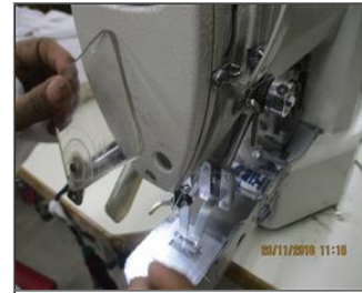
Photo of non-conformity 7.17 Eye guard of bartack machine was displaced .JPG
