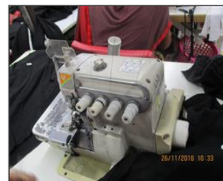
Photo of non-conformity 7.17 Eye guard of overlock machine was displaced .JPG
