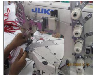
Photo of non-conformity 7.17 Eye guard of flat lock machine was displaced .JPG
