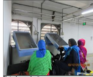
Photo of non-conformity Finding 7.3-Thread sucker machine operators were not using ear muff.JPG
