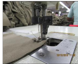
Photo of non-conformity Finding 7.17_Needle guard found displaced.JPG
