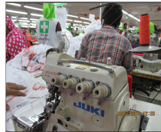
Photo of non-conformity Finding 7.17_Eye guard found displaced.JPG
